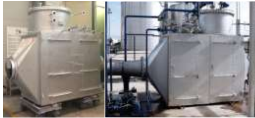
Counter Flow 2 stage 520 kW HRSG 12 Bar steam with water pre-heater for Anaerobic Digester
