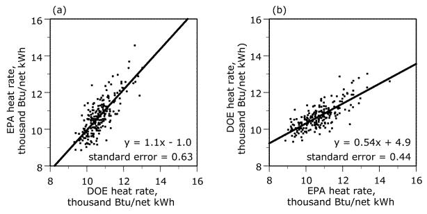
Figure 2. Attenuation bias due to EPA measurement error is shown in (b) where the EPA heat rate is used to predict the DOE heat rates. Points show annual (2009) plant-level heat rates. Data are from Quick (2014, supporting information) and EPA (2018).
