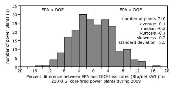
Figure 1. The differences between heat rates determined from flue gas measurements (EPA data) and fuel consumption measurements (DOE data) differ by  $\pm 11\%$  (two times the standard deviation) for 210 U.S. coal-fired power plants during 2009. The percent difference was calculated according to: 100 x (EPA – DOE) / maximum (EPA or DOE). Data are from Quick (2014, supporting information) and EPA (2018).
