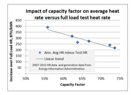
The graph below using USDOE/USEIA data shows the strong relationship between the decrease in EGU plant efficiency and plant capacity factors.
