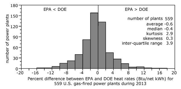
Figure 3. The differences between heat rates determined from flue gas measurements (EPA data) and fuel consumption measurements (DOE data), show a non-Gaussian (fat-tailed) distribution for 559 U.S. natural gas-fired power plants during 2013. The percent difference was calculated according to:  $100 \times (EPA - DOE) / maximum (EPA or DOE)$ .
