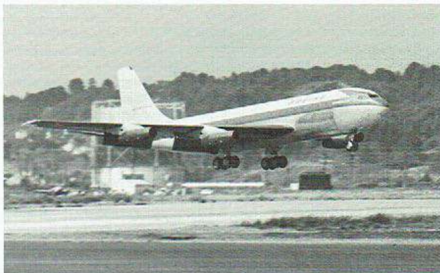
Prototype Boeing 707, the United States' first jet-powered transport, lifts off on its initial flight on July 15, 1954, under the power of four JT3 engines. This aircraft, known as the Dash-80, was presented to the Smithsonian Institution in 1972.
