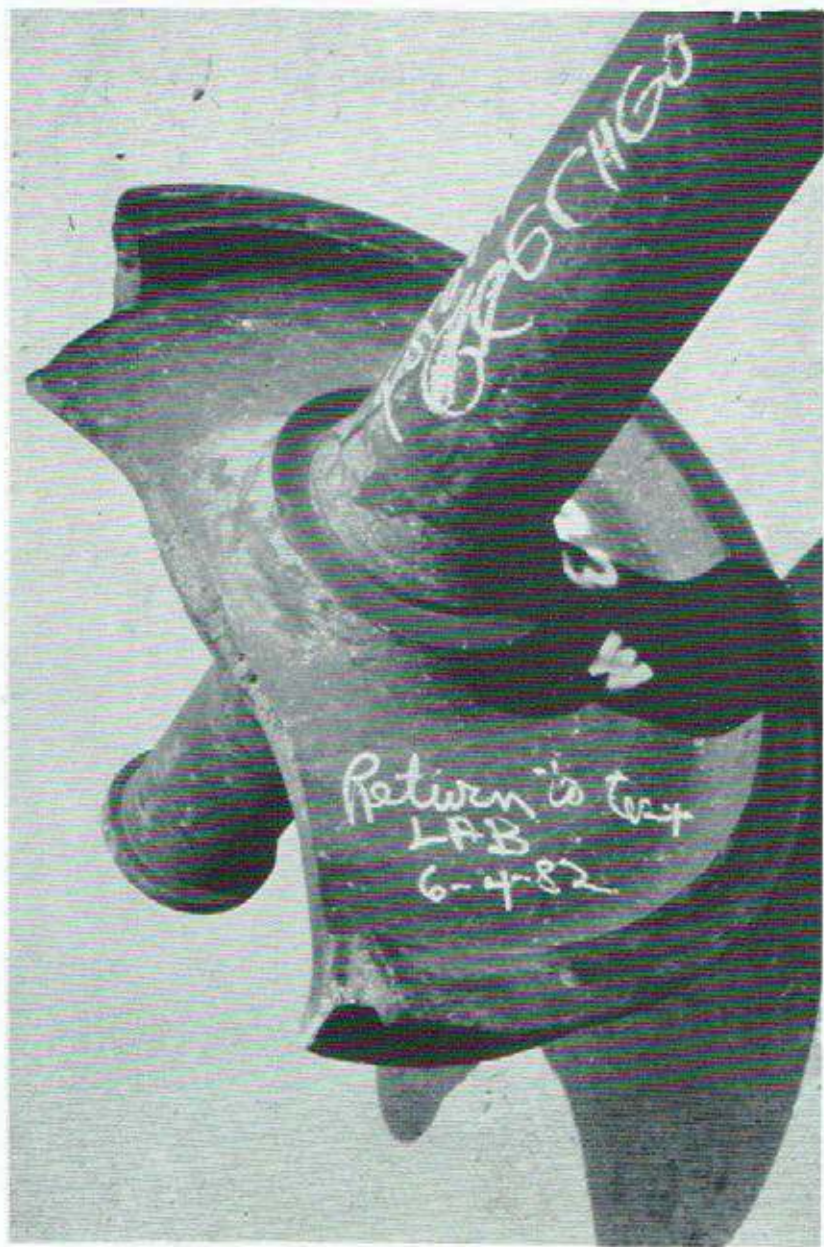
FIGURE 1. Straight plate steel freight car wheel which fractured in service due to thermal stresses developed by on tread braking.
