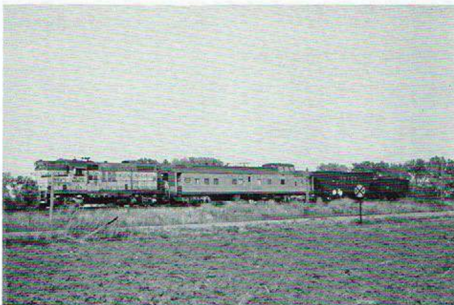
FIGURE 6. Union Pacific test train used to evaluate the effect of braking on railroad wheels.
