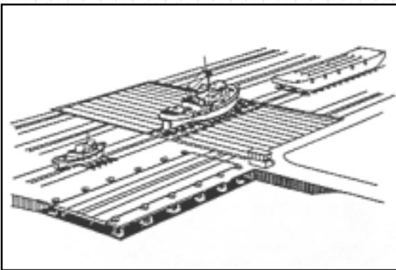
A transfer system can be added to a basic SYNCROLIFT® shiplift by providing railroad or crane-type rails on the platform and on the adjacent land area. The rails are arranged so that a transfer cradle, with a ship on it, can be rolled to the land area when the platform is at the yard elevation. The on-shore transfer system can be designed to permit movement in both directions.
