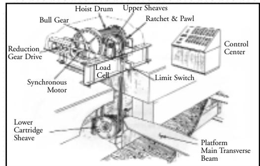
The electrical motors, used to drive the hoist, are designed to operate, up to a maximum required capacity, at a continuous fixed rate of speed regardless of load variations imposed by the distribution of the weight of the vessel. All of the motors are controlled from one central point. In the event of malfunction of any one motor, the entire system is automatically stopped.
