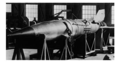
speeds of 3,500 mph. The word accuracy barely applied. In a 200-mile flight, the V-2 would miss its target by 10 miles.
