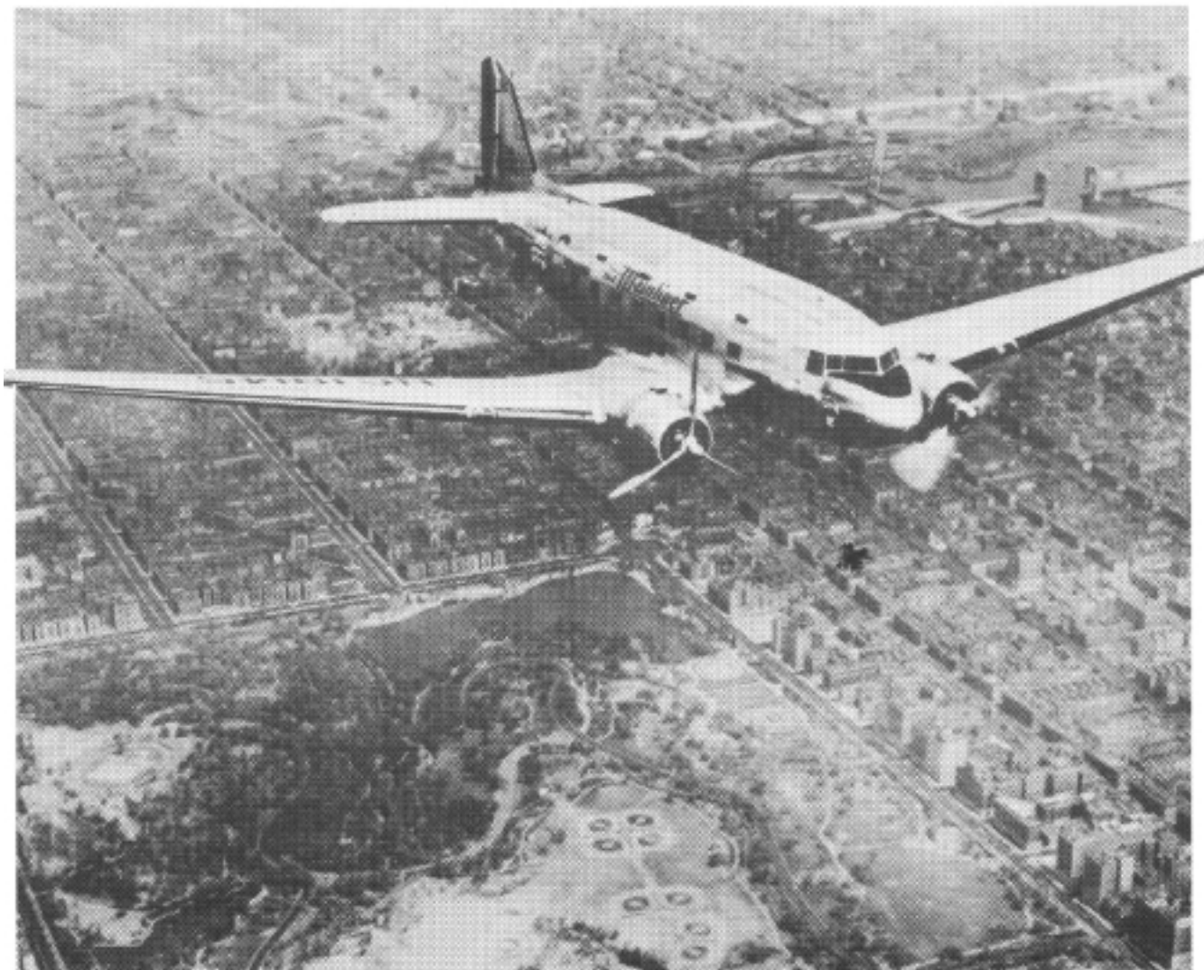
The first public demonstration of a feathered Hamilton Standard Hydromatic propeller, made by a United Airlines DC-3 over New York, N.Y., on April 6, 1938.
