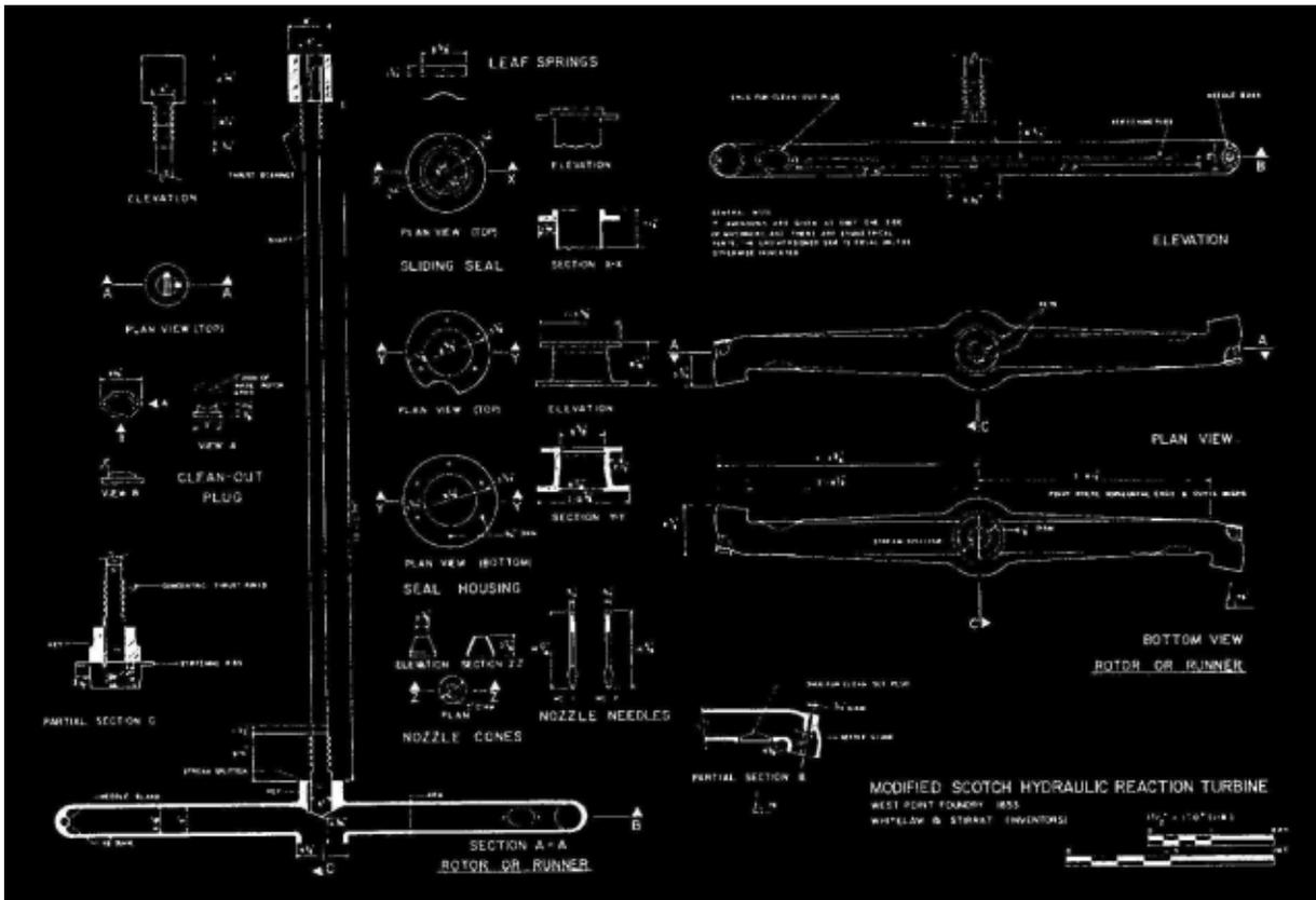
Of considerable concern was the efficiency value to be used. Since this value is a function of the nozzle and water jet velocities (and therefore the turbine angular velocity and the head of the water in the supply stand pipe) a fixed average value of 0.6 was selected for calculation purposes.
