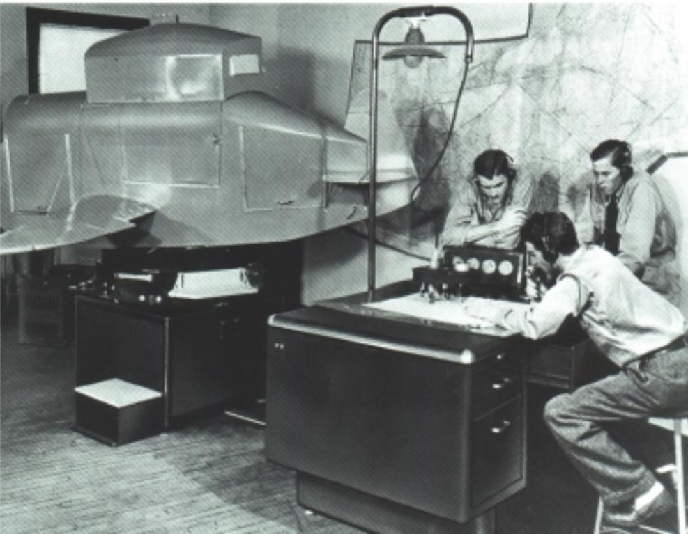
Figure 2: Instructors carefully watch the progress of a pilot using the Link Trainer
