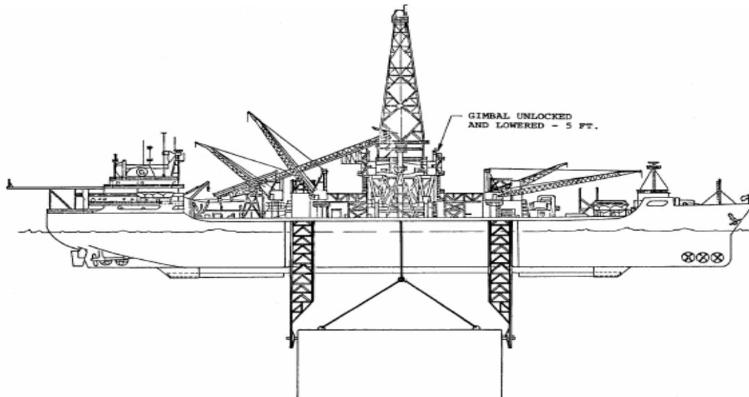
**SUBSEA EQUIPMENT LOWERED TO RELEASE DEPTH**
