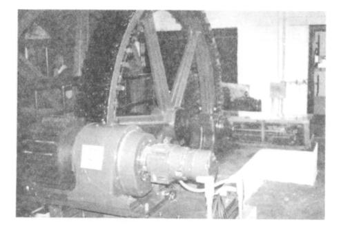
Wooden toothed drive gear with cable drum (left) and traveling-nut limit switch (right) Duquesne Incline
