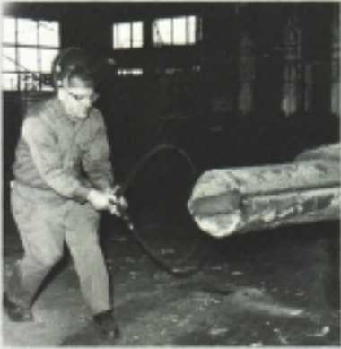
Steel alloy in finish forge operation. Shown is spindle, used with box beam in Rockwell's B- 1B. (1983)
